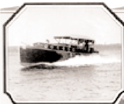
This boat powered with 200 h.p. high speed light weight motor. Makes 52 mph.
