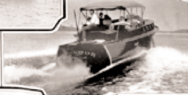
This boat powered with 200 h.p. high speed light weight motor. Makes 52 mph.
